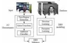
The flowchart for real-time AU recognition system
