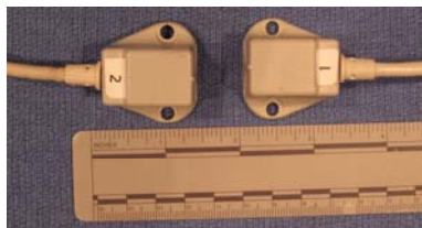
Figure 3: Flock of Bird sensors used as a six-degree of freedom electromagnetic tracking device.
