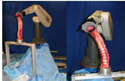
Figure 6: The PUMA 6 DOF robot replicates active voluntary motion of the entire thoracolumbar spine from data collected in vivo . Neutral and right lateral bending of an intact specimen are shown.
