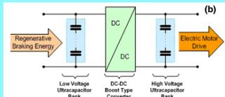
(b) Ultracapacitor based regenerative braking energy storage system in hybrid electric vehicle
