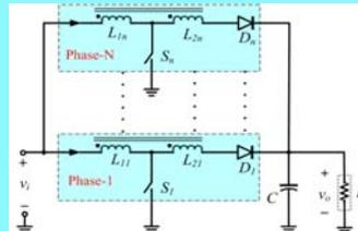
Proposed interleaved coupled-inductor boost converter.
