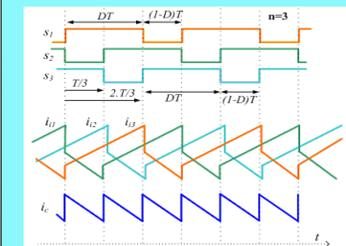
Output capacitor charging current of the interleaved converter.
