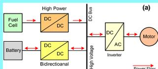
(a) Fuel cell based hybrid electric vehicle
