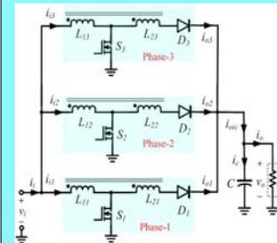
Coupled-inductor boost converter with the proposed boost converter clamp
