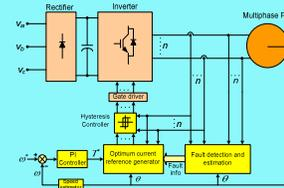
Block diagram of the proposed optimal fault-tolerant control scheme for an n-phase PM drive.
