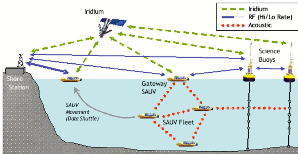
**Figure 8. Adaptive sampling within a mixed sensor fleet.**
