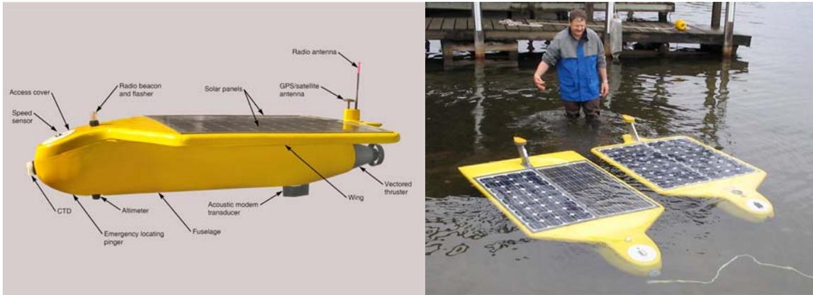
**Figure 1. Solar-powered AUV (SAUV) platform.**
